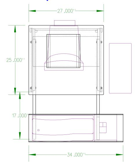
Typing Stand Computer Desk **Plywood Layout** Sketch #3 **Keyboard Shelf** Second Cut Top Top 25.000'' First Cut **Stand** Back Side Side **Third Cut** Shelf -29.750'--29 .750'-
