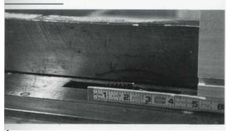
**1** To match the 2" height of the scrollwork, the groove must stop  $2^3/8$ " from the top of the end panels. The extra 3/8" provides for the 3/4" top minus the 3/8" groove cut into that top.
