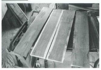
1 Matching figure and color is the first step. Here, two walnut boards with sapwood edges are being matched.
