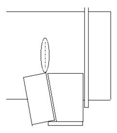
Make the jig out of 3/4" plywood, the length can be any convient size to accommodate scrap material on hand, to use it lodge material into angled notch, set fence on table saw to cut width of shim, this can be from sharp pointed to wider with blunt end. After each cut flip material over end for end to keep the material parallel.
