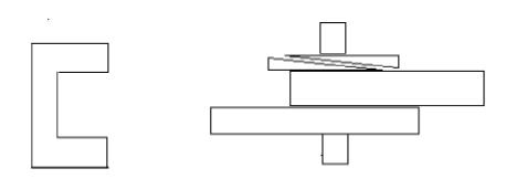
You can make a C- clamp by cutting a notch out of a rectangular piece of plywood, use wedges to lock material in place.
