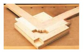
A simple clamp can be made for gluing up picture frames or other miter joints. Fasten a square to one corner of a base and add two strips to the opposite outer edges of the base, cut four wedges to lock the stock in place.
