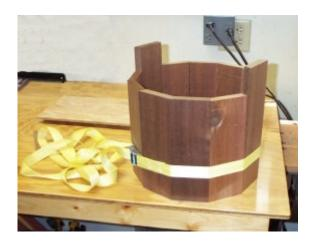
Next I routed dados which would give a nice groove for the black banding that would later be applied to "sit" in . I used a 3/4" straight bit in my router table. I adjusted the fence so that the top of the dado would be 1 1/2" from the top, or bottom when the stave is flipped. I set the depth to 1/8". The inside of the bucket has a 1/4" deep dado, 1 1/2"
