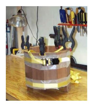
Jim Barry, at <u>Woodworkershop.com</u> gave me this tip: Lay out a width of wax paper longer than the bucket is round. Lay down 2 or 3 strips of masking tape sticky side up, on the wax paper. Lay the staves on the tape, the outside of the stave facing down. Apply glue to all edges required. Start to "roll up" the staves. When you have 3-4 rolled up, add the bottom (if one is required in the plan) and continue to roll up. When done, add your web clamps and let dry.
