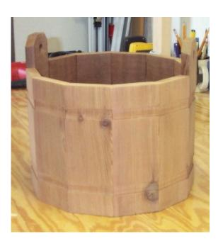
Trim the corners off the two 11" staves. I marked my diagonal line 1" in from each side and 1" down from the top. That gave me a little triangle shape I snipped off with the miter saw. Drill a centered hole 1" from the top of each 11" stave with a bit of appropriate size to accommodate the size of rope you will use for the handle.
