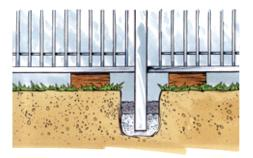
Secure the posts into position by filling the hole with wet concrete mix to a depth of 600mm. Then tighten all the tek screws firmly, checking line and level as you go.
