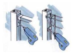
First, lay the panels and posts out along the fence line. Work outwards from the gate post and be careful to keep approximately 75mm ground clearance under the panels. Tek screw the panel with the fittings to the post. For wire-based fencing use U-Clips.
