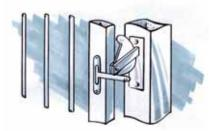
Firstly, position the 'D' latch on the post with tek screws so it will be aligned with the striker bar when the gate is closed. Then fix the striker bar to the vertical gate frame and check for smooth operation.
