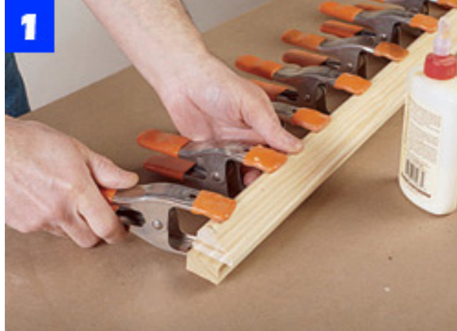
After gluing a 1/4 -in.-thick lath to a 3/4 -in. backer, add the molding to the lath. Use spring clamps to apply pressure.
