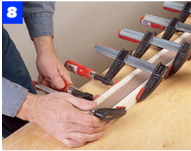
Clamp maple strips to both edges of a walnut field to form Frame 4. Make sure the pieces are flush on the back.
