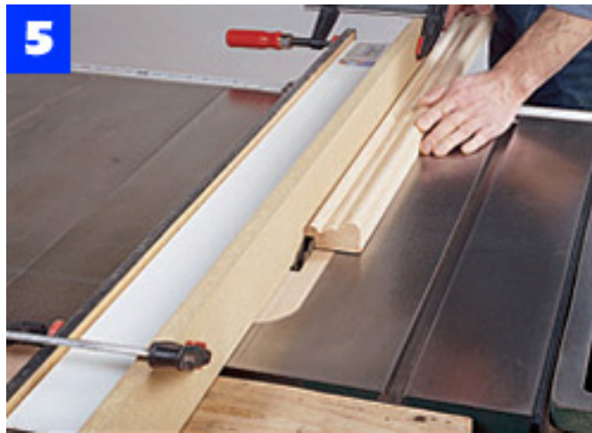
Frame 2 uses two moldings glued to 1 x 3 stock. Cut the frame rabbet with a dado blade and table saw.
