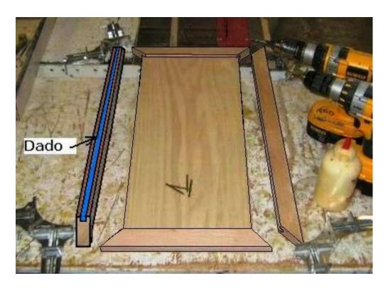
**Step 3: Make and Attach the Cabinet Doors** - Select the 3/4" Solid Oak Material and Plywood
