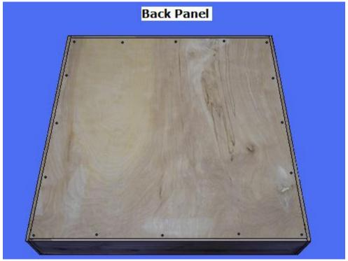
**Step 2: Cut and Assemble the Face Frame and Back Panel** - Select the 3/4" Oak Material and 1/4" Plywood
