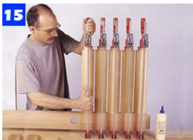
Multiple subassemblies are made in assembling the tabletop. First, slats are joined to the center rail.
