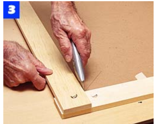
Temporarily nail the rear frame pieces together, and use a utility knife to mark the shoulders of the half-lap joints.
