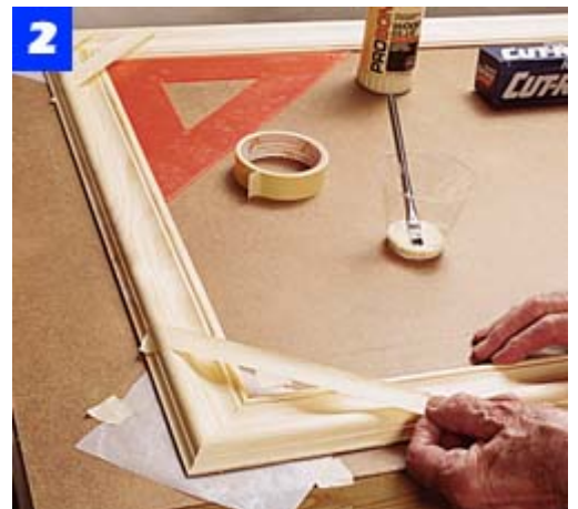
Apply glue to the miter faces and tape the pieces together. Use a drafting square to ensure the parts meet at 90°.
