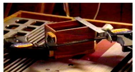
Dry assemble your box and holding it together with some light clamp pressure, measure carefully for the width you need to cut your top and bottom. Oversize your top and bottom if you're unsure of
