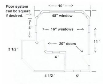
**Step 2:** Measure, cut and frame the walls per the drawings. Wall height is 7'. Most window opening will fit between 16" stud spacing. Use standard framing techniques, including a double top plate.
