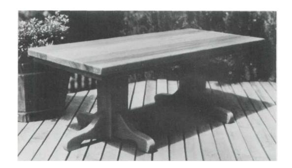
Here is a basic table design that can accommodate many uses. The table shown in the photo was made of redwood and assembled waterproof alue galvanized fasteners. Because it was designed to serve as a deck table, it is somewhat low in height. However. you easily can other substitute woods. use standard glue and fasteners, and raise the column height a few inches to create a handsome reading or dining table for the interior of your home.
