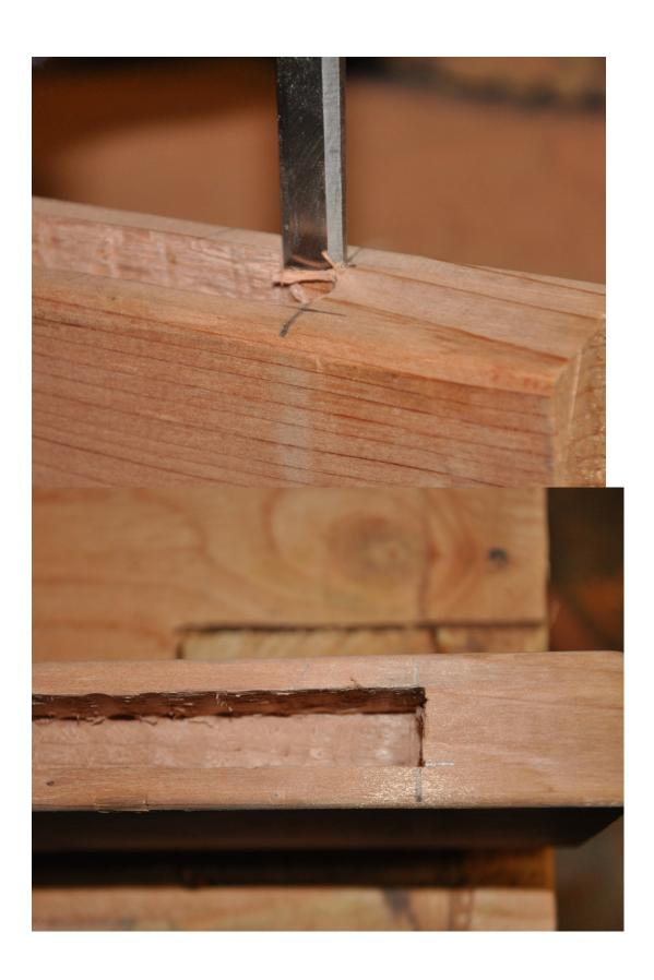
Use a sharp 3/4" beveled chisel and mallet to remove the remaining material. Keep the walls flat and make sharp  $90^{\circ}$  corners at both ends.
