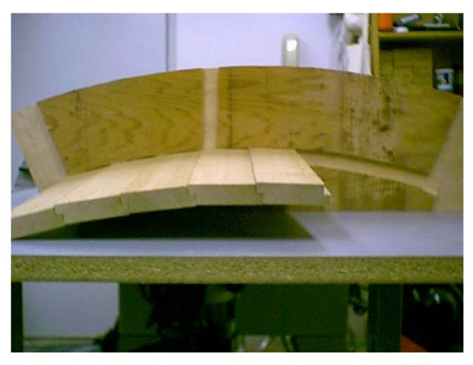
As you go around the wheel you will come to the 2x4 spokes. This is where it gets tricky. At each spoke you will need to custom cut each bottom piece to fit around the spoke. You also need to cut the opposite end in a mirror image so when we mount the other wheel side it will fit.
