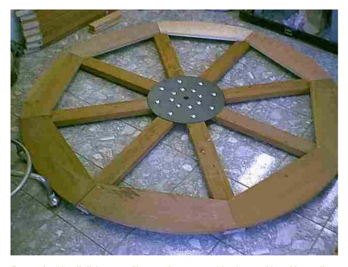
Go around and install all the screws. I hope you have a power driver because this could get really old really fast by hand. Now repeat the process for the other side.
