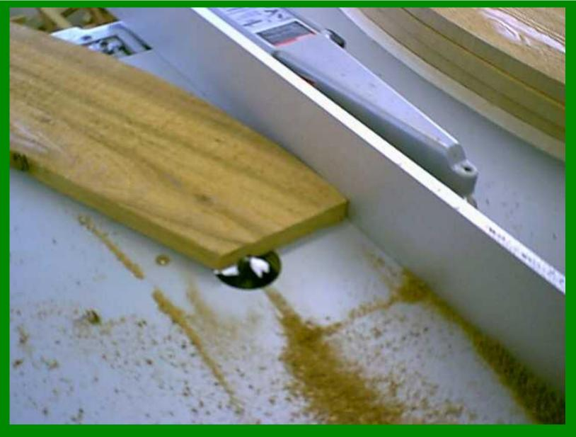
Once you've cut the slot you need to dado the notches where the 2x4 spokes and the 3/4" paddles will go. The spokes will fit half on one segment and half on the other so you will dado a 1 3/4" slot, 1/4" deep, completely across the segment.
