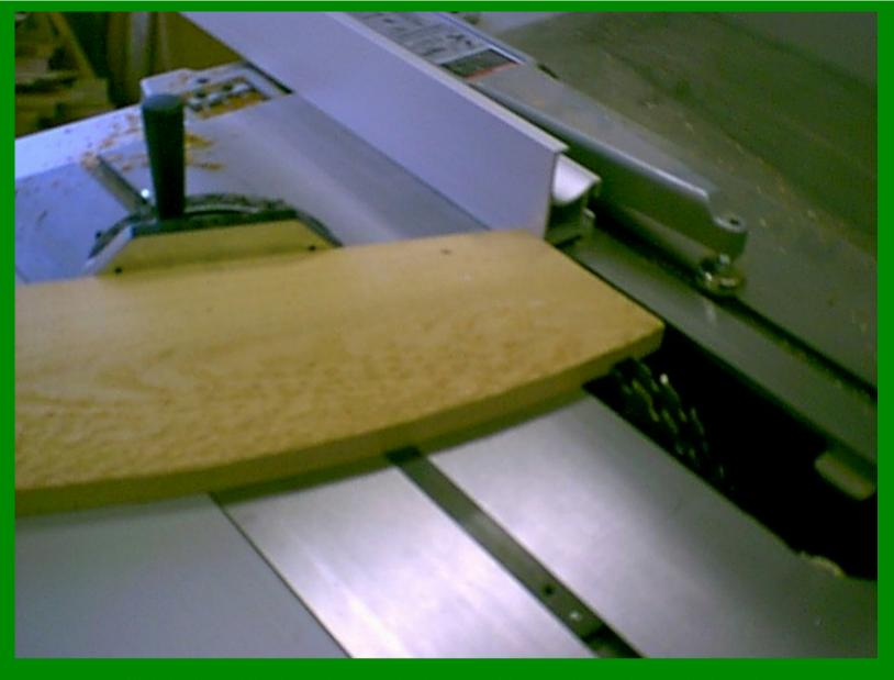
Next you will dado the paddle slots. These need to be 3/4" wide, 1/4" deep and cut only through the routed slot, not all the way through the segment. These paddle slots should be spaced evenly with one paddle butted up against a spoke and the other halfway in between. I kept the same angle for the paddles all the way around so they matched the spokes.
