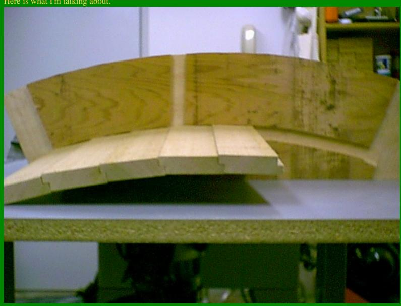
You want to set up the router with a fence so that you can follow the curve of the segment. Set the router to 1/4" depth using a straight cutter. Set the fence so that the notch will come close to the bottom of the segment on the end. I had to reset the fence and make a second pass because my router blade was only a half inch. The slot needs to be a little bigger than the thickness of the boards so they will fit on a curve.
