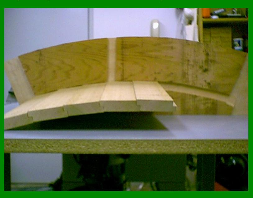
We are going to cut out the bottom boards that are really simple. I want to make my 5 1/2 foot diameter waterwheel about 12 inches wide so I cut them 11 inches long and 2 3/4 inches wide.
