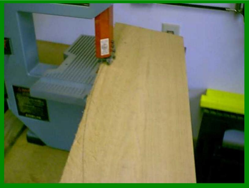
I used the paper template I made from my computer layout to draw the radius on top of each segment. Next you'll cut the to radius. You can use a band saw,saber saw or cut them by hand.
