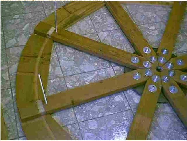
Place the bottom boards in the slot that goes around the wheel overlapping each one. Actually these should be in place from the last step.
