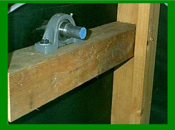
I marked the shaft while I had it in place so I would know where to weld the wheel. I put the shaft through the wheel hub and welded it in place.
