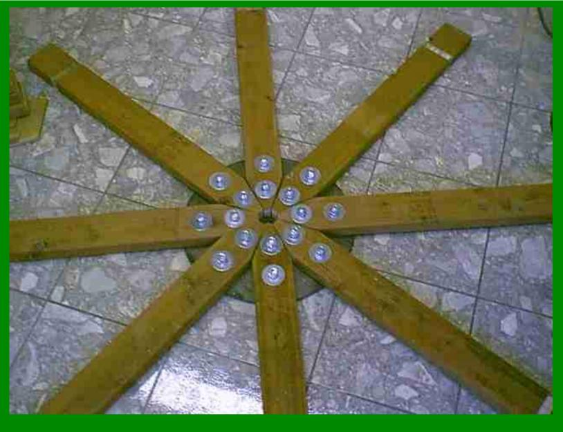
DO NOT tighten the nuts yet, just make them finger tight. The spokes need to be loose so you can make some fine adjustments. I laid it out flat on the floor and with a tape measure, measured from spoke to spoke to get them as evenly spaced as possible.
