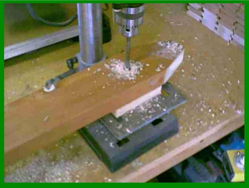
Next we countersink the holes to accommodate the square portion of the bolt that will stick through the hub.
