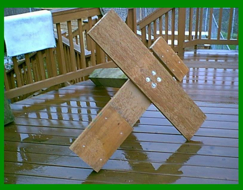
I used four really long lag bolts and washers to mount the timber to the base. I added a piece of 2X4 and 2X12 to each end of the base to make it level.
