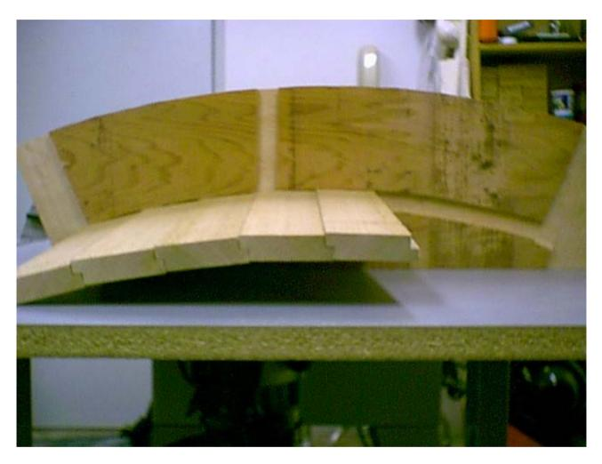
Take the opposite side of the wheel and carefully place it onto the threaded rods to help line things up. Start pushing the bottom boards that are sticking up into the slot around the top wheel. Line up the spokes as close as possible by looking through them to the other side.
