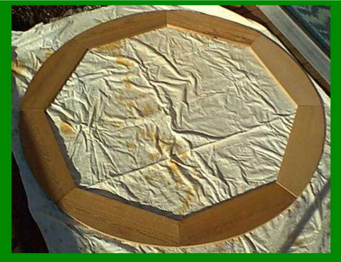
Once all the pieces are cut, lay them out and make sure that they fit well together and there are no large gaps between segments. If there is a gap you can go back and re-cut them but make very tiny adjustments.
