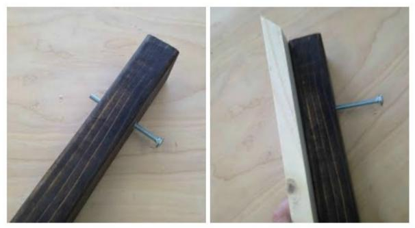
**B.)** Place a bolt through the top hole, and then hit lightly with a mallet, this will leave an indent showing you the exact location of where the receiving end of the bolt should be placed.
