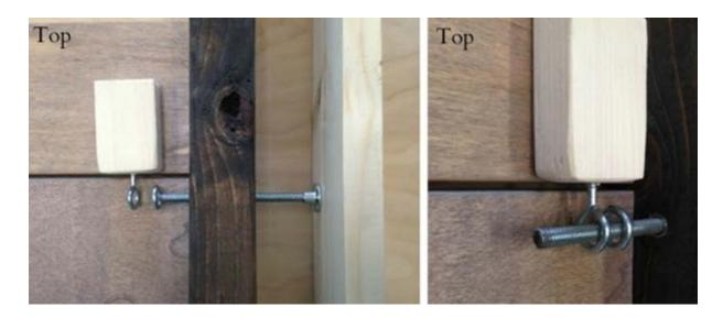
Note: The eyelet on the upper lid (the second one featured above) is not entirely necessary. If the trim piece you attached to hid the gap is secured well, it will prevent the upper lid from opening until the lower lid is unlocked. When making this I did not realized that the trim would hold it in place as well as it does. However, if you are concerned about it being more secure, add the extra eyelet hook for peace of mind.
