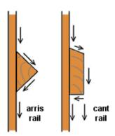
Traditionally arris rails had tongues cut at their ends which fitted into slots cut in the posts. The tongues took the full weight of the forces on the fence, so they often broke after a time.
