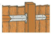
Unless the boards are going to be fitted between the posts, it is simpler to use cant rails (with their vertical back edge) and fix them across the front of the fence posts.
