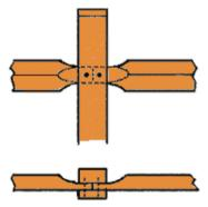
Galvanised steel repair brackets, which are available in a number of designs to suit both arris and cant rails could be used to repair broken rails as necessary. These repair bracket can be used when constructing a new fence, they avoid having to spend a lot of time cutting the tongues and slots.
