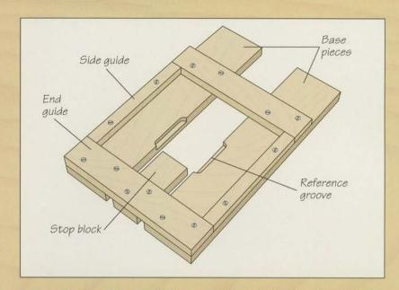
the stock thickness. Then, with the router positioned inside the guides, grip the tool firmly, turn it on, and lower the bit into the workpiece. Guide the router in a clockwise direction to
