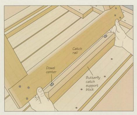
3 Installing the dowels
