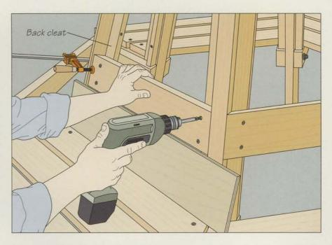
With two double frame sections positioned on opposite sides of an ash tree, a tree bench apron is fastened in place. Since the bench was built in the shop and disassembled for easy transport and positioning, installing the remaining pieces—the seat and back slats, the cap rails and the last apron—is a simple matter. The boards can be fitted into position and the screws driven into their predrilled holes.
