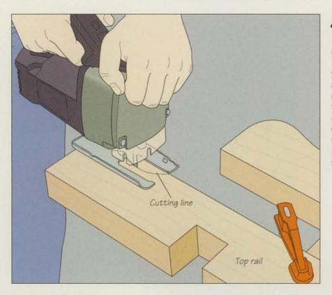
A Shaping the ends of the top rails
