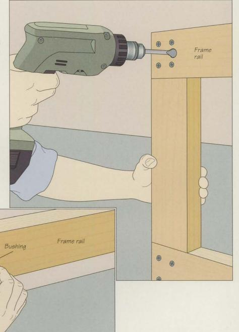
3 Installing the bushings
