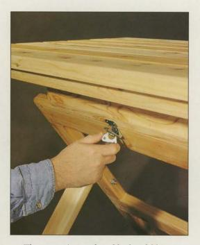
The convenience of a table that folds can be a liability when it is laden with food. One way to ensure that the table does not collapse at an inopportune time is to use a butterfly catch pull to lock the leg rail and support block together.
