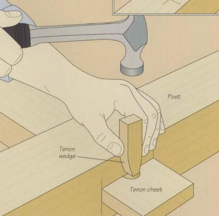
Assembling the posts and rails 4 Fit the posts and rails together and mark a line along the top of each cheek where the tenon emerges from the mortise. Disassemble the joint and drill a 1-inch-diameter hole through the tenon centered on the line. Cut a 1/2-by-1-inch hardwood piece into the bullet shape shown at left; make the length of the tenon wedge about equal to the post thickness. Slide the tenon into the mortise and strike the wedge firmly with a hammer until the joint is tight.
