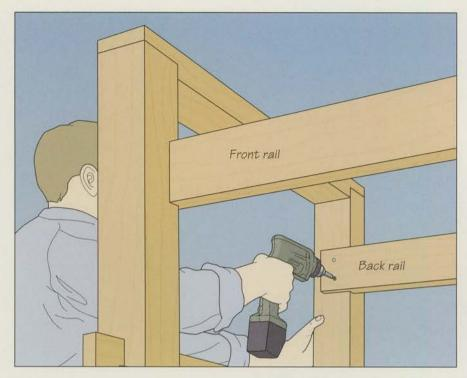
Attaching the front and back rails
