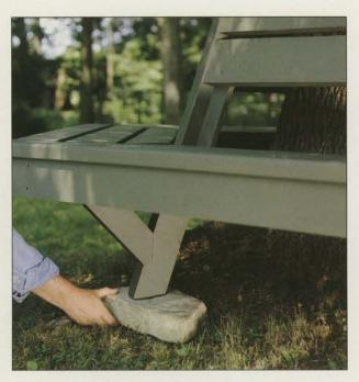
Rather than trying the painfully difficult task of cutting all the legs of the tree bench to fit uneven ground around a tree trunk, level it using flat rocks as wedges.
