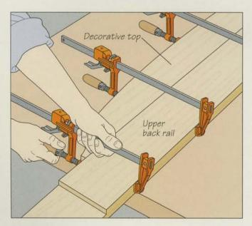
Decorating the top rail 4 Referring to the anatomy illustration on page 104, trace the shape of the decorative top on the stock and cut it to shape with a band saw. Then attach it to the upper back rail with glue and clamp the two pieces together (above).
