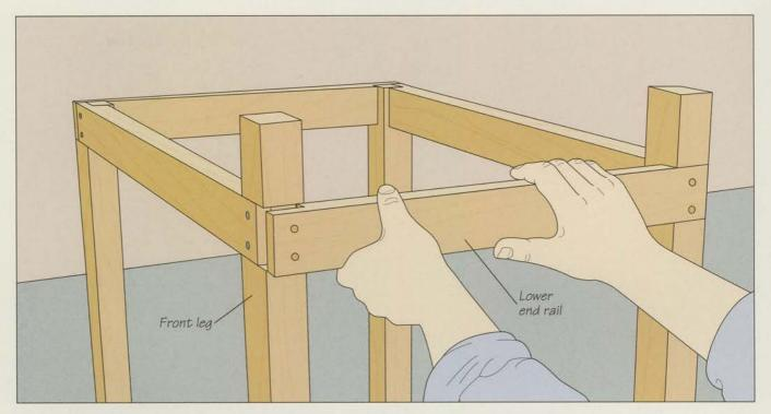
3 Installing the end rails
