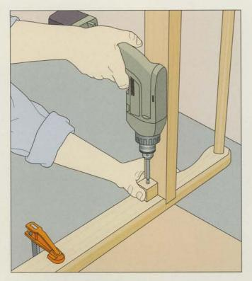
3 Attaching the support blocks and drill a %-inch-diameter Cut four 1-inch-square blocks and drill a %-inch-diameter Attaching the support blocks hole through each one. Glued and screwed to the handle rails, the blocks will support the slats at the front and back ends of the top. Clamp the top assembly on edge to a work surface
