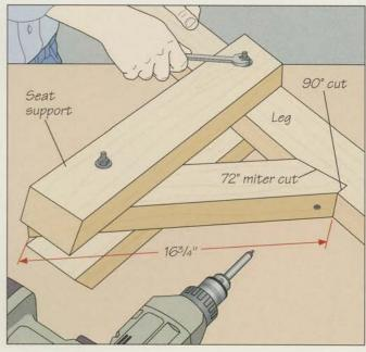
Assembling the legs, braces and seat supports
