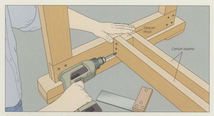
Attaching the center beams to the sides
