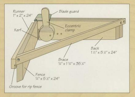
To use the jig, set it on the saw table in front of the blade with the runner and fence straddling the rip fence. Clamp the workpiece in the jig and position the rip fence to align the cutting mark on the workpiece with the blade. Feed the jig into the cutting edge. (Your first use of the jig will produce a kerf in the back.) Flip the workpiece around and repeat to cut the other cheek (below). Remove the jig to cut the shoulders.
