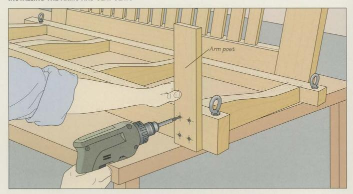
Attaching the arm posts . Position the arm post 2 inches from the end of the front seat rail flush with the bottom of the rail. Drill 4 pilot holes, then glue the arm post in place and secure it with screws (above). Repeat the procedure for the second arm post.
