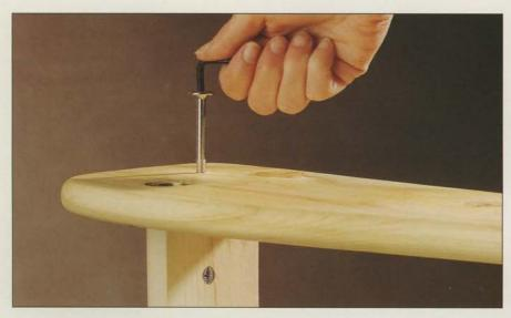
Cross dowels are commonly used in knockdown furniture, but their strength and durability make them ideal for outdoor furniture that is not designed to be taken apart. A cross-dowel connector is used to join an arm to an arm post in the chair shown above, providing a much stronger connection than screws could, and saving the task of fashioning a more elaborate joint.
