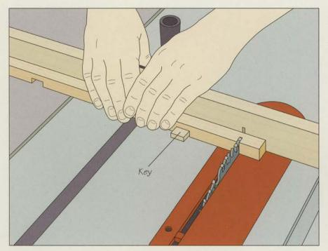
3 Cutting the lattice strips to length Once all the joinery cuts have been in the lattice strips, use the same setup to cut the pieces to length. Replace the dado head with a combination blade. For each strip, slip the last dado you cut over the key and feed the piece into the blade (left).
