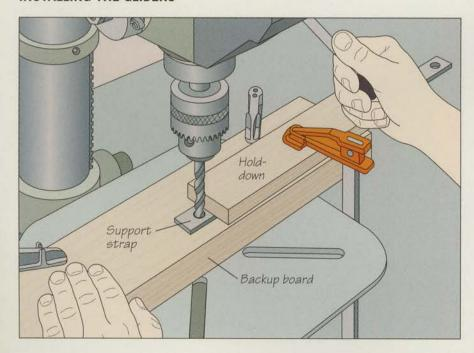
1 Drilling the holes in the support straps
