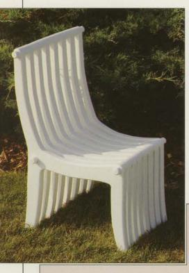
The curved chair featured in this section is built by joining eight identical H-shaped units with steel rods. Each unit is separated from the adjoining one by three 2-inch-diameter spacers—two at the rear leg and one at the front. The curve is achieved by using 1½-inch-long spacers in back and ¾-inch-long spacers in front.
