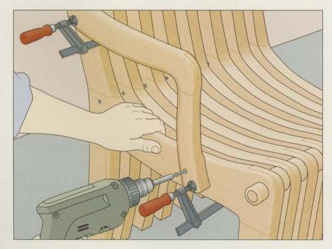
Attaching the arms to the chair 4 Attaching the arms to the Drill two clearance holes through each arm—one at either end—and apply glue to the flat areas that will contact the chair. Clamp the arm in position on the chair and fasten it in place (left).
