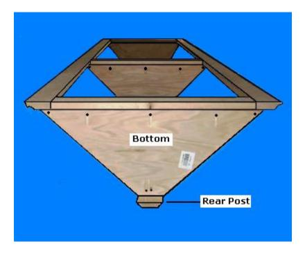
**Step 3: Assemble the Shelf Frame** - Select the Rear Post, Front Frame Assembly, the Top/Bottom Panel and Permanent Shelf
