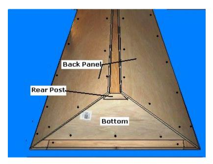
**Step 4: Make and Attach the Back Panels** - Select the 1/8" x 4' x 8' Plywood Panel
