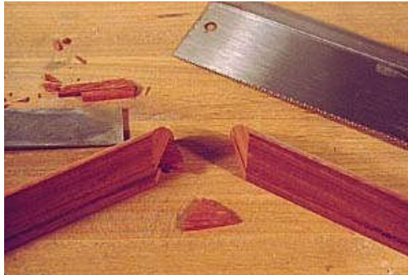
Photo 13- Fitting splines into the corner joints.
