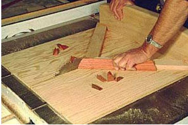
Photo 8- This table saw miter jig will cut very accurate joints for your tray. The jig is worth the effort to build well because you'll use it in the future for other cuts. Use a flat piece of plywood for the base, and carefully make and fit the runners on the bottom that ride in the miter gauge slots so that the jig slides smoothly with no side to side slop.
