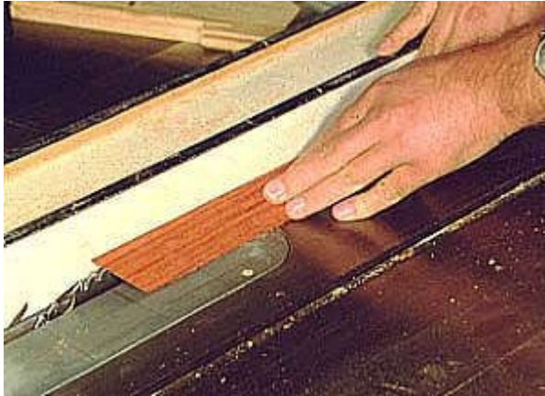
Photo 10- Deepening the kerf on half the ends for the splines.
