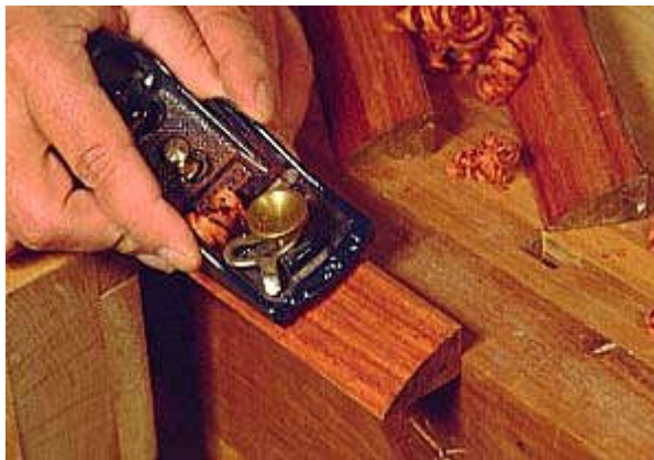
Photo 7- Rounding the lower area of the sides. Your block plane must be sharp to do this work effectively. A new block plane out of the box will probably not have the iron
