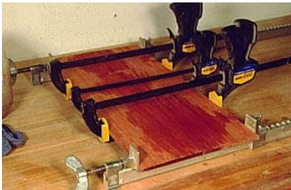
Photo 4- Edge glue the thin parts together for the tray bottom. The edges that get glued must be straight to get a good glue bond. If they are not straight, make numerous very small cuts on the edges of the boards at the table saw, flipping the board between each cut so the freshly cut edge rides against the fence for the next cut. This will gradually straighten the edges.
