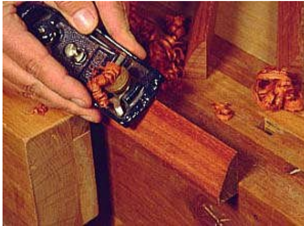
Photo 6- Using a block plane to round over the outside faces of the tray sides. If you don't have a block plane you may choose to leave the pieces with a flat bevel.
