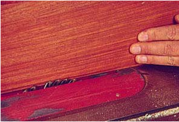
Photo 12- Cutting a rabbet on the lower edge of the bottom to leave a lip that will fit in the groove in the sides.
