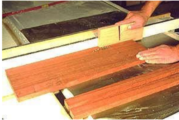
Photo 1- Rip out your parts. A push stick such as that shown here is a basic safety device for making cuts on pieces of smaller width on the table saw. Every woodworker
