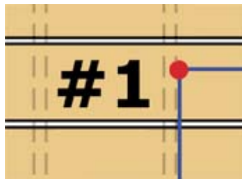
Image B: Notice here that the deck joist is located on the outside edge of the mark.
