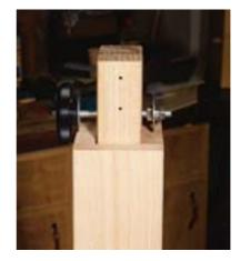
Some simple hardware from your local home center store allows you to lock the post solidly, but quickly loosen the post and readjust for any height. The hardware is shown at right, resting on top of the column before being attached through the holes.
