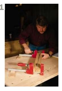
To form the post, the rough piece is ripped into three pieces, the center piece is cut to form two small blocks, and then the whole thing is glued back together. screwed together using butt joints. The slotted post supporting the top section is formed by cutting, then regluing the pieces – no complicated router work. The top is ½"-thick Baltic birch plywood pieces nailed together to form a torsion box for extra strength.
