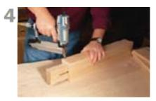
As you glue up the column, use the post to check the spacing. The post should slip easily into the sleeved column. You want the post to move easily, but don't make make it too loose or you'll make the stand wobbly.
