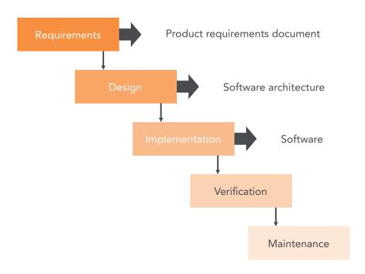
The waterfall approach is a kind of software development as we can see in the figure starting from requirements determinations to design then implementation and verification and finally to the maintenance process.
