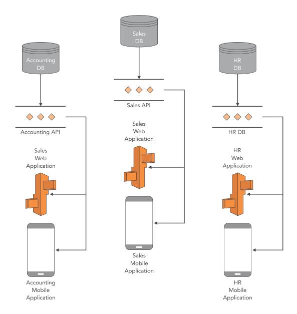
Here is an example of a micro service architecture diagram shows that 3 databases then integration with web and mobile applications from sales database as an example to sales web application, then to the mobile application as sinks receiving and sending to the server and API.
