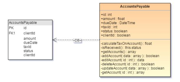
The previous diagram shows how the accounts payable is and its table which is the same structure as the accounts receivable table and class but they must be separated as deductive or additive amounts that must be in a separate processing areas.
