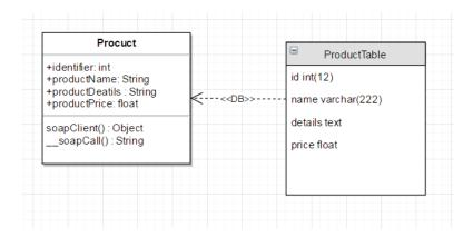
As we can see in the previous class diagram, we find that the product class on the left side is a class in PHP as an example that contains 4 class members or class variables and 2 functions. The class variables are reflected into our database table on the right side as 4 database table entities and the datatypes may differ from String (in our class on the left) to Varchar or text on the right.
