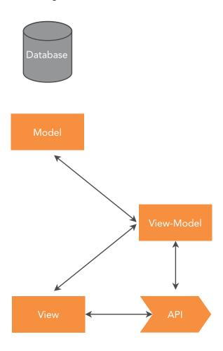
The diagram shows that the Model has all the database heavy lifting, then the view-model shows the connection between the view and the user interaction, to the model with the database, and comes the API as another alternative to the view in case integrating with another or external entity.
