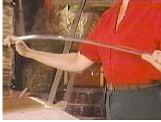
Polycarbonate tubing is more flexible than other types of tubing (i.e. acrylic)
