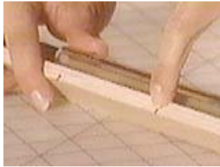
Measure and mark the jig at the drill points
