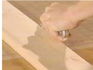
Use a piece of wood or other straight edge as a guide for the rotary knife
