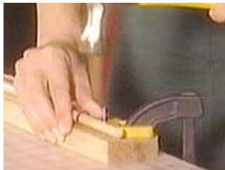
Drill holes in the ends of the dowel and nail them down to make a clamp
