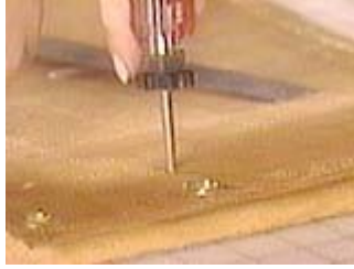
Push an awl through the screen and into the drill holes on the wooden jig
