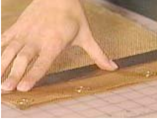
Mark screen with marker for placement of tubes and holes
