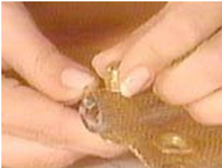
Slide the tube in between the layers of screen, line up the holes and install the hardware
