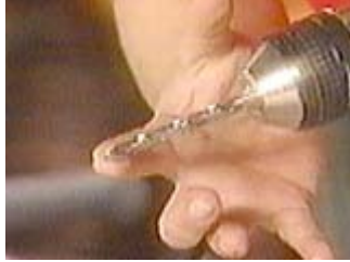
Drilling holes in plastic requires a special drill bit
