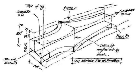
To make a suitable jig, cut two pieces 18 mm ply or MDF to 1180 mm long, the same length as the leg, and 72 mm± wide (Piece A above) and the other 90 mm± wide (Piece B above) Dry biscuit the edge of Piece A to the face of Piece B. Mark a line along the inside of the corner on piece B. Plot the outside profile required on Piece A. (Ignore the inside curve at the bottom of the leg.) The profile can be plotted directly onto the MDF, or a full size paper template attached. Cut and smooth the curves.
