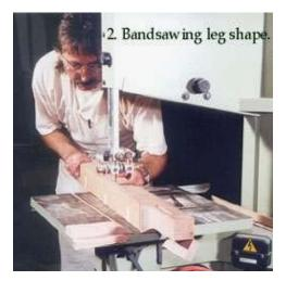
Bandsaw the waste from the legs. Cut one face, and re-attach the offcuts with masking tape. Cut the second face. Screw each leg back into the jig and use the spindle moulder, or a router and pattern cutting bit to follow the profile. Extra screws may be inserted to secure the leg in the jig, but screw only into the biscuited face; the holes will be hidden later. (These legs are from a different job, but the profile and procedure is the same.)
