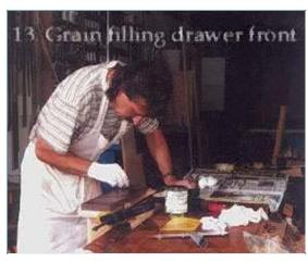
varnish, and 15% mineral spirits Third, and subsequent coats were cut with about 30% of both mineral spirits and alkyd oil varnish. It's wiped on, and buffed off fairly quickly, concentrating on one manageable area at a time.
