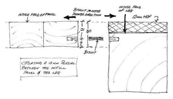
With this job done, the cabinet bottom can be trued up, cut to exact length, and dry biscuited to the inside faces of the side panels. In this cabinet there is a bottom front rail attached to the front edge of the cabinet bottom, and this may also be dry biscuited on, leaving this item 50-60 mm overlength at either end.
