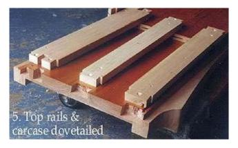
done at this stage, except that this is when the bottom rail is glued to the bottom shelf. Gluing at this point ensures that the rail overhangs the right amount at both ends.
