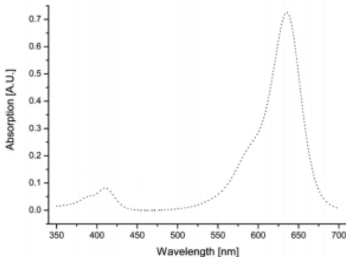
Figure 1. Absorption spectra of E131 (concentration of 4 mg/L).
